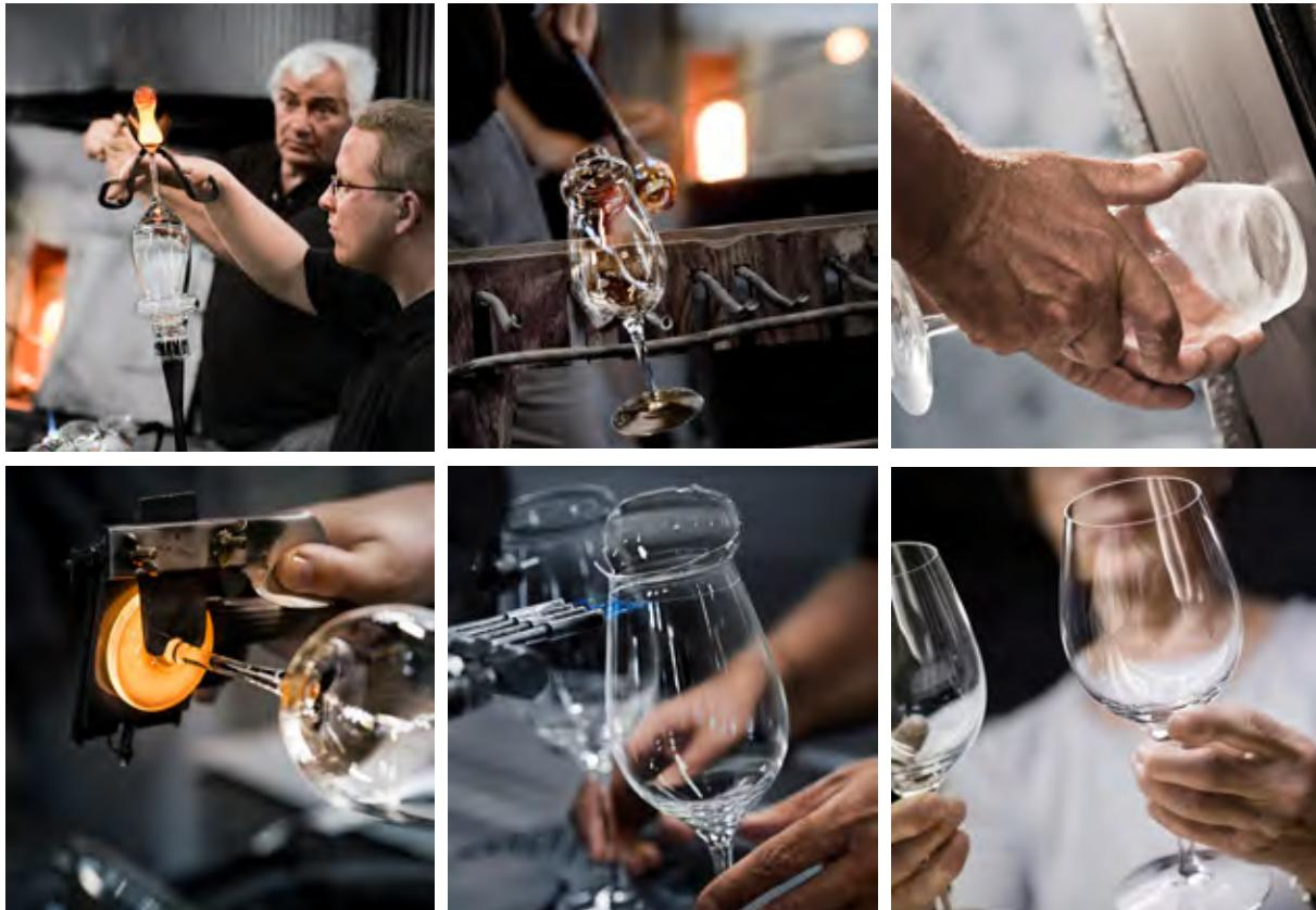
7. The assistant knocks the glass off the blowpipe using a special holder known as a carry-in-fork. The glass is then fetched by a carrier, who places it in a lehr, where it is slowly cooled. After cooling, an initial quality assurance check is carried out by a sorter. If the glass is deemed to comply with Orrefors' stringent quality standards, it is sent for further processing.
